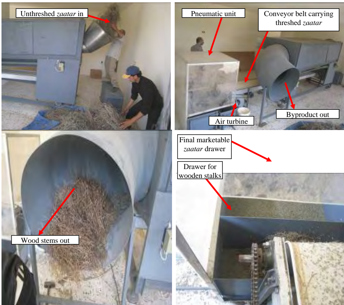
Figure 26. Operational trial of the ESCWA-pilot mechanical zaatar thresher
