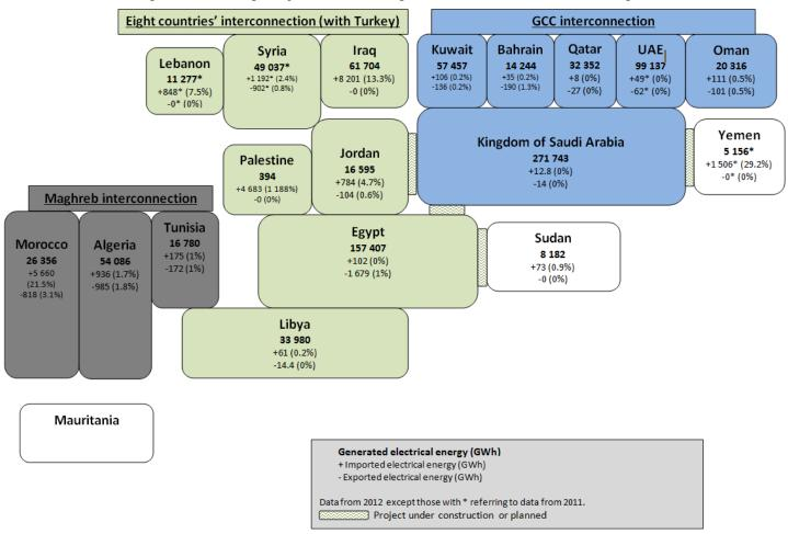
Figure 1-8: Existing and planned electrical grids interconnections in the Arab Region
