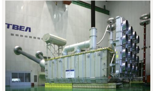
\pm 1100\text{kV}/650\text{MVA} converter transformer
