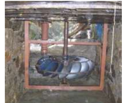
Improved Water Mill with Metal turbine and shaft
