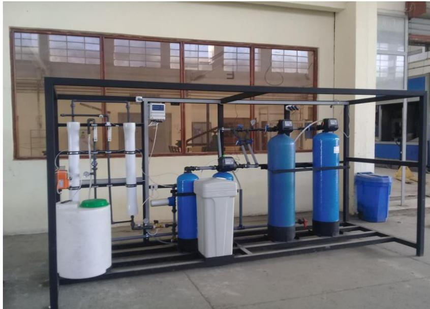
Pilot unit Hybrid process involving Ion exchange resin coupled with NF or RO
