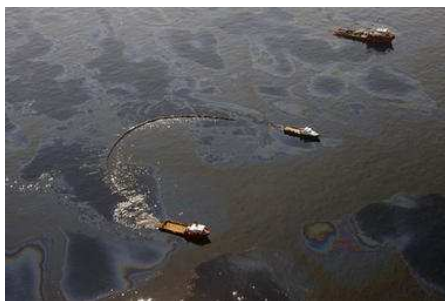
Work boats pull booms to skim oil at the site of the BP oil spill in the Gulf of Mexico (UPI/Newscom)
