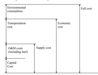
Figure 17. The full component costs of desalination
