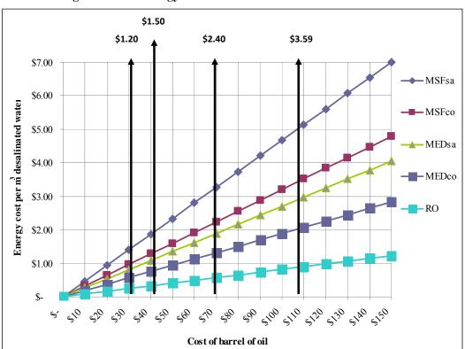
Figure 18. The energy cost of desalination in relation to the cost of oil
