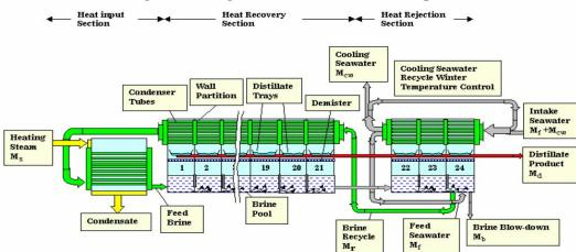
Figure 15. Diagram of the MSF desalination process
